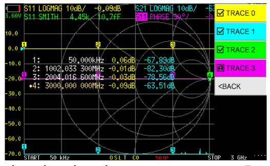
Tap on **[TRACE n]** (e.g., **[TRACE 2]**) will open and activate TRACE 2, and an **[A]** marker will appear ahead of "TRACE 2". Tap on another menu item (e.g., [TRACE 3]) will open and activate TRACE 3, at this time, an \( \bar{\text{A}} \) marker will appear ahead of "TRACE 3", and the \( \bar{\text{A}} \) marker ahead of "TRACE 2" becomes ✓, which means TRACE 2 and TRACE 3 are both opened and TRACE 3 is current active.
