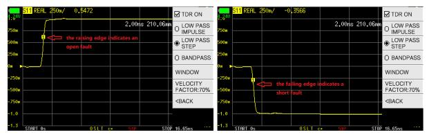
**LOW PASS IMPULSE** is another signal processing mode for cable fault detection.
