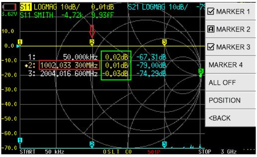
Tap on [MARKER n] (e.g., [MARKER 2]) will open and activate MARKER 2, and an ☐ marker will appear ahead of "MARKER 2". Tap on another menu item (e.g., [MARKER 3]) will open and activate MARKER 3, at this time, an ☐ marker will appear ahead of "MARKER 3", and the ☐ marker ahead of "MARKER 2" becomes ☑, which means MARKER 2 and MARKER 3 are both opened and MARKER 3 is current active.
