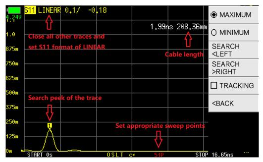
To get the cable length value, please open the menu 【MARKER】 → 【SEARCH】 → 【MAXIMUM】 to move the marker to the peak of the trace, and the estimated cable length will be displayed on the screen.
