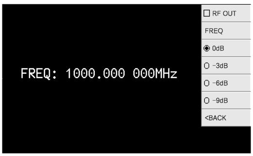
**(RF OUT)**: Turn on/off the RF output.
