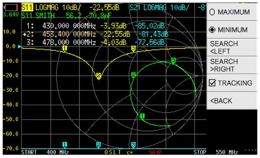
**【TRACKING】** is used to automatically track the maximum or minimum value of the trace. As shown in the figure above, if you want MARKER 2 to automatically track the minimum value of the S11 LOGMAG trace, firstly you should activate MARKER 2, and then tap on **【MINIMUM】**, and finally turn on **【TRACKING】**. After doing that, MARKER 2 will automatically move to the valley point of the S11 LOGMAG trace after each sweep.
