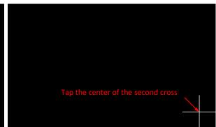
**Note:** After completing the calibration of the touch screen, you **MUST** execute saveconfig command to save the calibration data.
