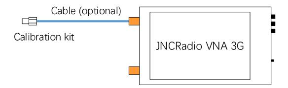
Tap on **[OPEN]**, the device emits a beep, and the menu turns gray and is inoperable. Wait for letter "O" appears at the bottom of the screen, indicating that open calibration is finished.
