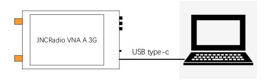
Important Note: Only USB-A to USB Type-C cables can be used for charging and data transfer.
