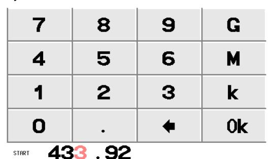
The virtual keyboard includes numeric keys, backspace key, unit key, ok key.
